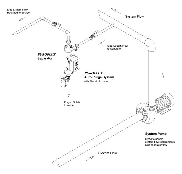
Pressure differential across system pump must be great enough to produce proper flow in separator
